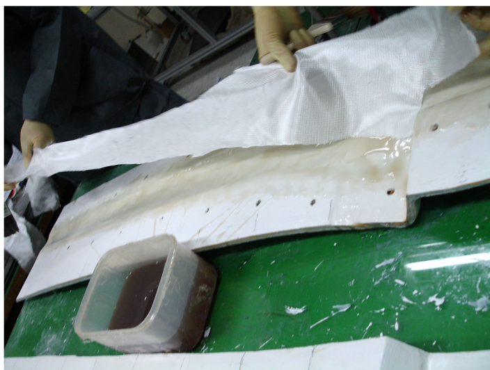
Figure 19. Lay-up process on the mold. This figure is published in color on http://www.ingentaconnect.com/content/vsp/acm
